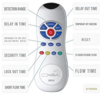
The Remote Control is available for easy maintenance of extensive installations requiring custom settings.
